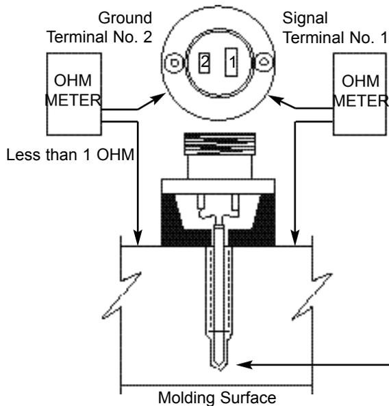
All MoldMonitor sensors may be tested with an OHM meter. Check resistance across terminals from terminal No. 1 to ground.
