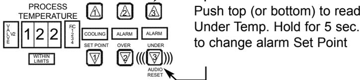
Note: Alarm span will remain when cooling set point is changed
