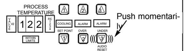
Note: Audio will automatically re-arm when temperature reaches set point
