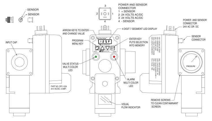
Note: Input CAP may be reversed with pressure gauge.
